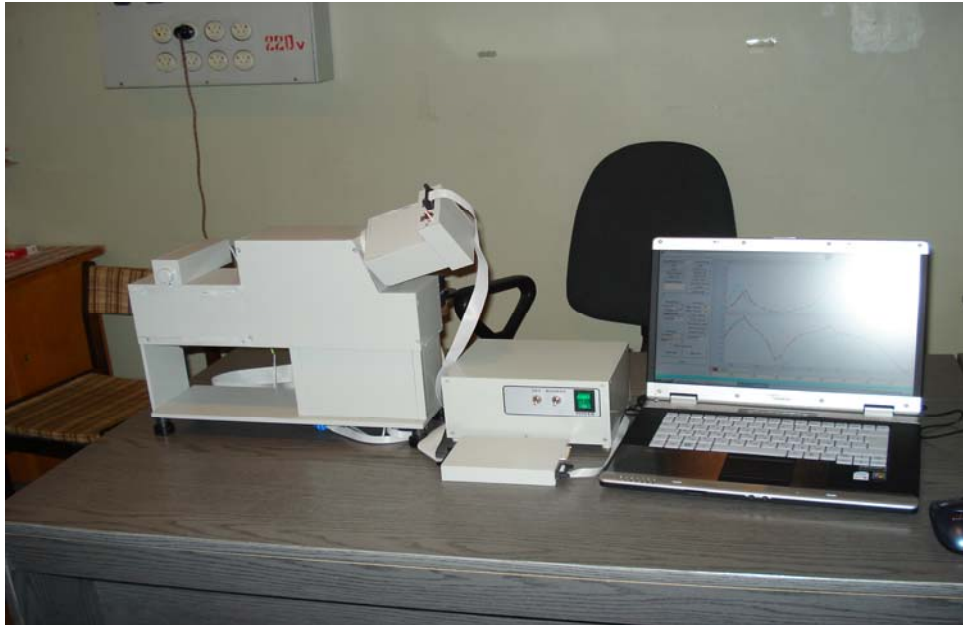
Figure 1: High precision real-time multi-wavelengths spectroscopic ellipsometer with binary polarization modulation (one of modifications) with registration and recognition system at the base of notebook
